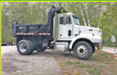
2001 Peterbilt 330. CAT 3126 250Hp, 9 Speed Eaton RT8709B, 33,000 GVW, Air Trac Air Ride, 3.90 Ratio, 10' Steel Dump Body, Auto Tarp, 200K Miles, One Owner and Driver, Clean Pre-Emission, No Headaches, $28,500.
