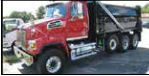
2018 WESTERN STAR TRI AXLE DUMP. DETROIT DD13, 505 HP, Allison Auto, 20K/46K/20K Tuff Trac Susp, #MJG7789
