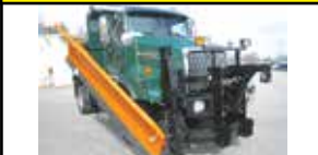
2016 Western Star 4800SB. All Wheel Drive, 10' Monroe Dump Tip Spreader body, 11 plow & 11' wing, Detroit DD13 #MHN3427
