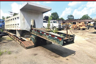
1980 GENERAL LOWBOY: 35 Ton, Detachable, Ground Bearing Lowboy, 19' 9" x 8' Deck. Independent Gas Motor For Neck, Needs Some Decking, Pony Motor For Wet Line. As Is. Dump Body Not Included, $3,500
