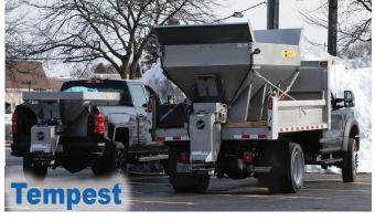
Available in chain drive or with the new Helixx shaftless auger system
