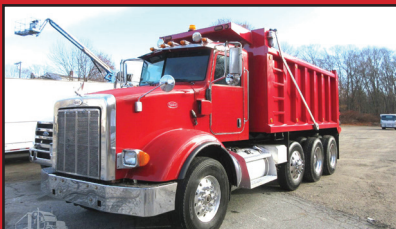
2011 PETERBILT 365 TRI-AXLE 6x4 DUMP. Cat C13 6 Cylinder 12.5L Diesel 335 HP, Allison Automatic, 16540 FA, 59500 RA, Air Ride Cab, PTO, Wet Kit, 16' 5" x 5' 3" Steel Body, $84,900
