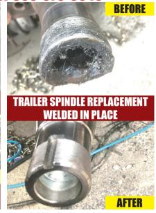
• Drive Spindles From 1 Ton To Class 8 Trucks • Trailer Spindles From 3,500# To Class 8 Axles Spindles can also be repaired by welding up the worn area and then remachining to factory spec.
