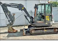
**9540 2022 VOLVO ECR50F.** Coupler, 3rd Valve, Dig Bucket, Hyd Thumb, Rubber Tracks, 166 Hours, **\$63,500.**
