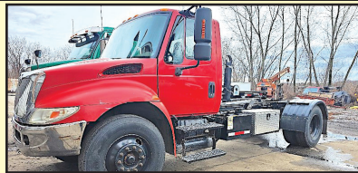
2004 IH 4300, DT466, AUTOMATIC, AMERICAN HAS200 HOOK- LIFT, 36" JIB HEIGHT, 20K CAPACITY, PINTLE WITH FACTORY AIR-TO-REAR, 342K MILES, RUNS PERFECT, FRESH BRAKES AND SERVICE. HOOK CANNOT BE MADE ADJUSTABLE. $25,000
