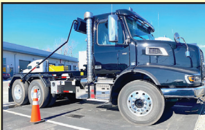
NEW VOLVO SHORT WB TANDEM AXLE ROLL-OFF: D13- 425HP, 13 SPD, I-SHIFT TRANS. 66K GVW, PALFINGER AMERICAN ROLL-OFF, 40K HOIST W/ EXT. TAIL OPTION, PIONEER COVERING SYSTEM. HOIST DOES UP TO 16" CANS. TRUCK CAN BE SEEN AT DARIO DIESEL, WORCESTER MA.
