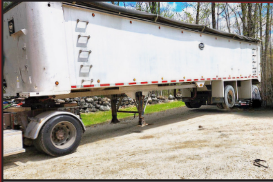
2010 MAC TRAILER MFG. 40 Ft Tandem Axle, Not Road Worthy - Front Axle Displaced, 40 Ft, 72" High, Hendrickson, Air Ride, Tandem Axle, Frame-Less, Very Fixable, $12,000.
