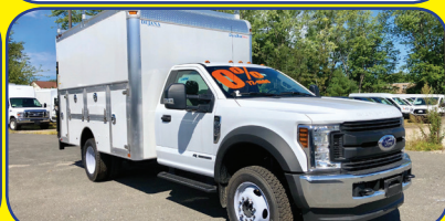
2019 FORD F550. Diesel, Auto, Power Group, 16' Duracube Max Utility Van Body w/ Aluminum 1600 lb Lift Gate, #07397
