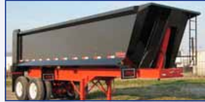
NEW 2010 SCHEIN 26' STEEL DUMP TRAILER, HARDOX 450, TANDEM AXLE, SINGLE PT., 11X24.5, HIGH-LIFT GATE, 60" SIDES, IN STOCK NOW
