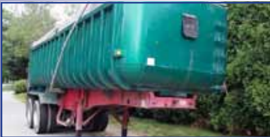
1994 FRUEHAUF: Reyco suspension, 26'L x 96"W 54" inside height, 24.5 tires, all steel wheels, fixed tandem axle. Super clean only hauled asphalt. Manual tarp system. 30% tires, 50% brakes. Please call for more information.
