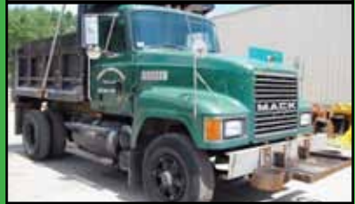
1996 MACK CH612: 6 WHL DUMP, 12K FRONT, 23K REARS, 10' STEEL BODY, PINTLE W/ AIR, 3 SHUTES, MACK SPRING RIDE, 5 SPEED, MACK EM 7, 275 HP, 205K MILES, STK# 580, $16,500
